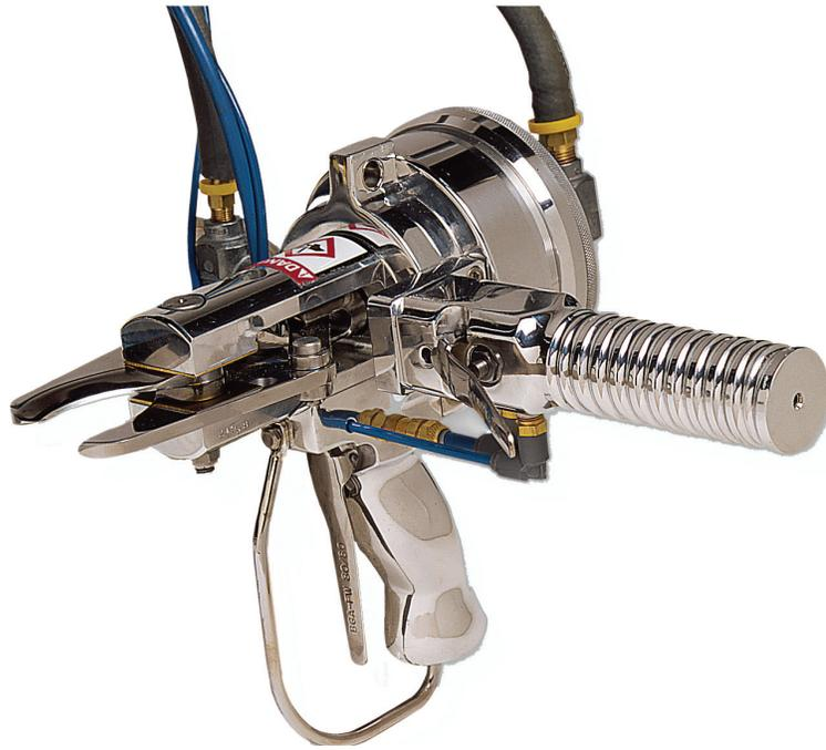
**The Jarvis Model TBC - pneumatically powered cutter for cutting beef tongue bones.**
