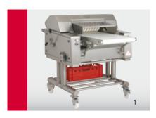
The multi-purpose BXM is suitable for derinding of thicker flat meat cuts. The material to be derinded can be put on the infeed conveyor in unsorted positions. The product to be derinded is precisely introduced to the blade due to a special pressure device that automatically lowers the infeed conveyor.
