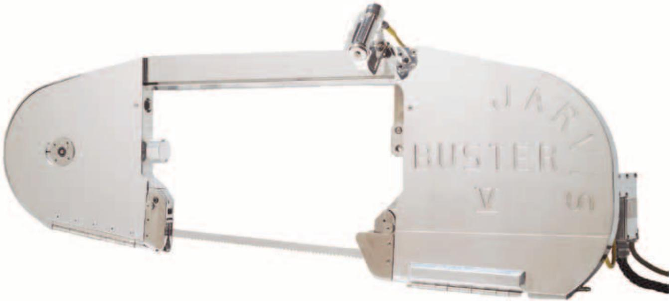
**The Jarvis Model Buster V - electrically powered bandsaw for splitting bulls, cows and horses.**
